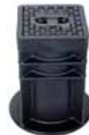
Series 80/33-01 Surface box for service connection valves to DIN 4059 Fixed height Body of PA+ Lid of cast iron
