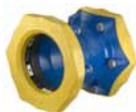
Series 631/70 Supa Maxi™ universal tensile straight coupling DN 50-300 PN 10 Ductile iron
