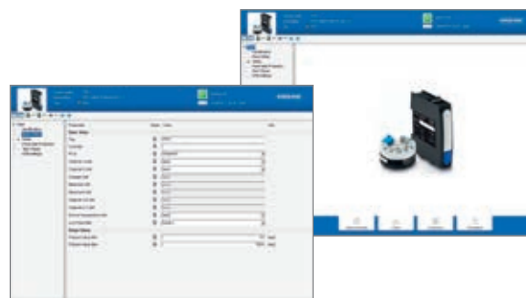
Configuration of OPTITEMP TT 51 temperature transmitter via PACTware™
