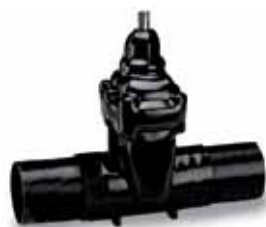
Series 46/70 Gate valve with long spigot ends DN 50-600 PN 16 GS-C 25 N With external PUR coating
