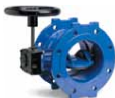
Series 756/1 Butterfly valve Double eccentric Double flanged Integral seat IP 67 gearbox DN 200-2800 PN 10/16 Ductile iron
