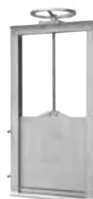
Serie 772/7172 Channel penstock Uni-directional up to and incl. 1000 X 1000 mm, bi-directional in larger sizes With non-rising stem Stainless steel AISI 304 200 x 200 mm - 2000 x 2000 mm
