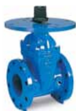
Series 45/59 Flanged gate valve with post indicator flange DN 100-300: 250 PSI DN 350-400: 200 PSI Ductile iron UL/ULC listed, FM approved
