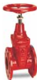
Series 06/35 Flanged gate valve with position indicator DN 50-400 PN 10/16 Ductile iron VdS approved (DN 50-200 only)
