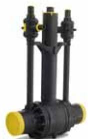
Series 85/50 Ball valve with spigot ends, stem extension and 2 purge points DN 50/Ø63 mm - DN 150/Ø180 mm PN 10 PE 100
