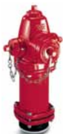
Series 27/00 Dry barrel fire hydrant Modern style Bury depth 2 ½' - 10' 250 PSI Ductile iron UL/ULC listed, FM approved
