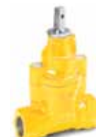
Series 03/25 Service connection valve with internal thread DN 25-50 PN 4 Ductile iron With external epoxy coating
