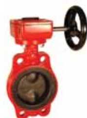
Series 75/31 Butterfly valve Centric with fixed liner Semi lug DN 50-300 PN 10 /16 Ductile iron VdS approved
