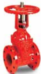
Series 45/56 Flanged gate valve with rising stem DN 65-300 250 PSI Ductile iron UL/ULC listed, FM approved
