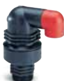
Series 701/40 Combination air valve DN 20, 25 and 50 Threaded BSP \frac{3}{4} ", 1" or 2" PN 16 Reinforced nylon
