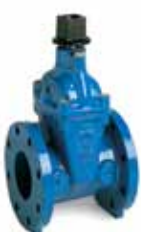
Series 45/59 NRS Flanged gate valve with wrench nut to AWWA C509 DN 100-300: 250 PSI DN 350-400: 200 PSI Ductile iron UL/ULC listed, FM approved
