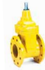
Series 06/70 Flanged gate valve Short DIN F4 DN 40-600 PN 10/16 Ductile iron With external epoxy coating
