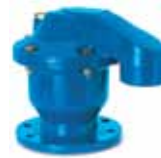
Series 701/30 Kinetic air valve Inlet flange DN 50-300 PN 16 Grey cast iron
